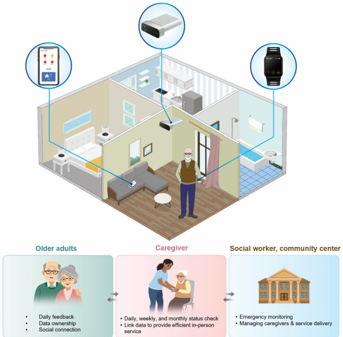
Figure 1. Community-mediated digital health platform architecture for vulnerable older adults. The 3-tiered service delivery system enables comprehensive health monitoring and care coordination. At the individual level, older adults in their homes interact with smartphone apps, smartwatches, and motion sensors for continuous health monitoring. When personalized algorithms detect health deterioration signals, assigned community caregivers provide targeted support through phone calls or home visits. For severe health declines or emergencies requiring coordinated response, the system escalates to the community center for comprehensive intervention. This hierarchical architecture ensures appropriate care intensity while maintaining older adults’ independence in their home environment.
