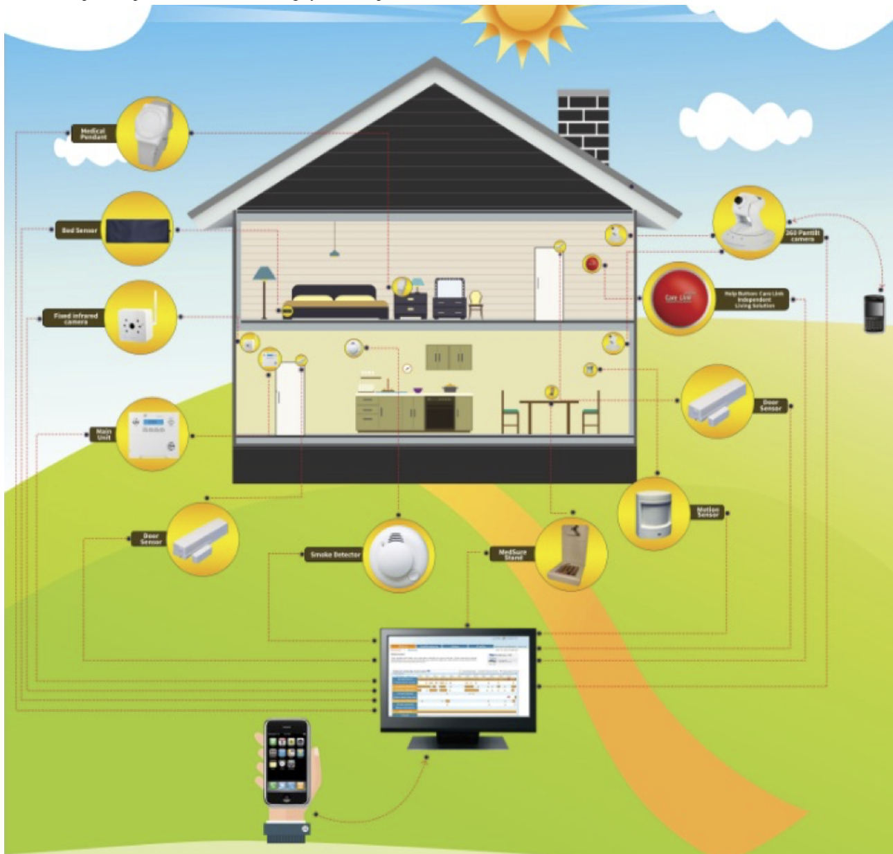
Figure 1. Example of a passive remote monitoring system setup.
