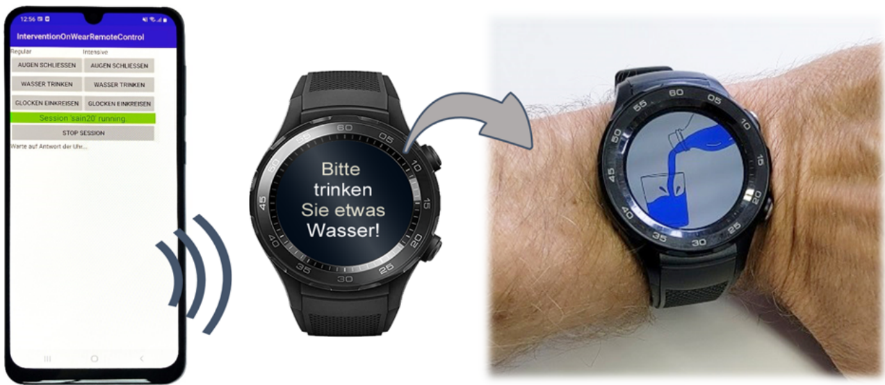
Figure 3. Images and embedding of the applied prototype—smartphone with an app to manually trigger interventions on a watch, which is mounted on the patient's wrist, showing instructions (in this case, "Bitte trinken Sie etwas Wasser," which means "please drink some water").
